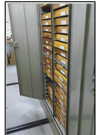
Figure 1. ANSP cabinets are compressible to save aisle space © Jeff Freeman.
