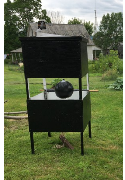
3 x 3 ft. box trap at Galick Farm. The black beach ball provides reflected, polarized light attractive to tabanids. Photo: Jeff Freeman
